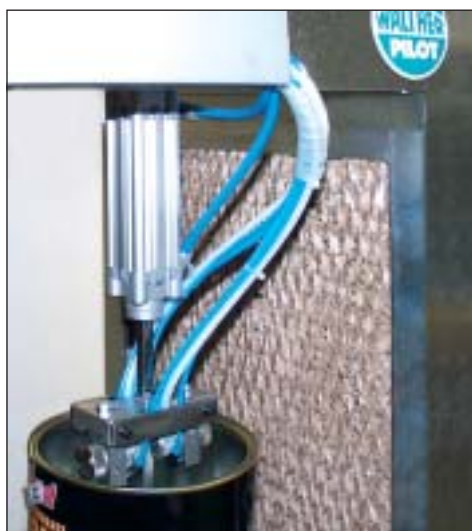
Compact spraying system with two guns on a lifting cylinder and multi-layer filter mats.
