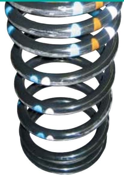
Multi-colour marking of components
