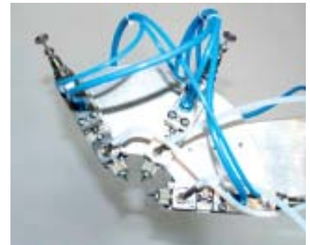
Gun arrangement for multi-colour marking
