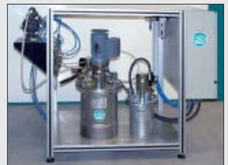
Compact system for small application quantities with pressure tanks for the coating material and solvent as well as a double diaphragm pump and a flushing gun.
